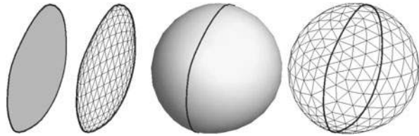
Fig. 9.10 The results of least-square meshes ( left ) and our non-linear solution ( right ) for a planar curve
