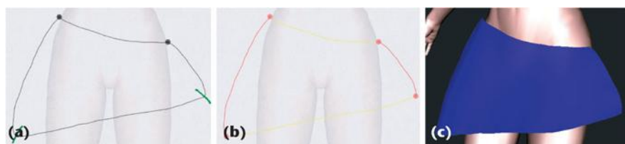
Fig. 14.3 a Lucy drew in contour mode the outline of the skirt without sharp corners at the bottom, and the corner-detector failed to put breakpoints there, she therefore gestures (overdrawn in green here) to indicate the need for new breakpoints, in the form of short strokes that cross the contour. b The new breakpoints have been inserted. c The reconstructed skirt
