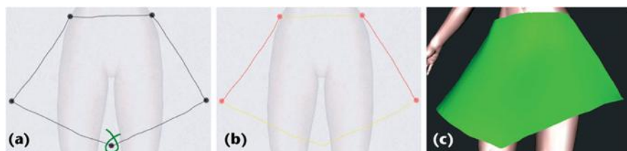
Fig. 14.2 a Lucy has drawn a few lines to indicate the shape of the skirt in contour mode ; the corner-detector has detected a breakpoint that she does not want. Lucy makes a deletion gesture (a curve in the shape of an \alpha enclosing the mistaken point) to delete it. b The breakpoint is deleted, and the lines have been classified: the silhouettes are in red and the borders in yellow. c The surface inferred by the system once Lucy requests a reconstruction
